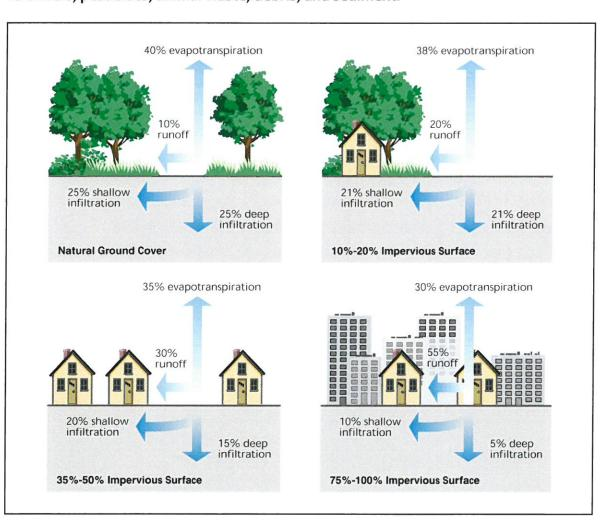
As illustrated in the diagram above, the amount of stormwater runoff increases as the amount of impervious surfaces increases. Poorly managed stormwater runoff can cause a variety of problems such as environmental degradation and localized flooding.
